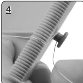
Line the wire up with a groove on the other side, then wrap it around the second button.
